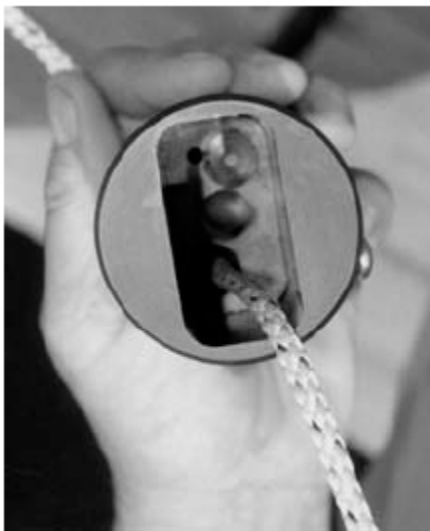
Rope halyard fed into HTF (bottom view)
