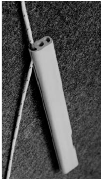
Inserting FF4 ferrule into top of luff
